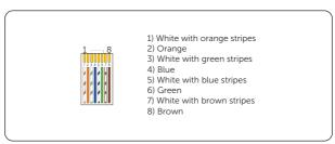
Figure 8-35 Pin of COM terminal
