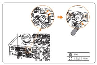
Figure 8-33 Connecting to the inverter
