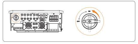
Figure 9-5 Turning off the lockable DC switch
