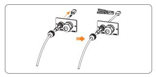
Figure 8-32 Installing the RJ45 terminal
