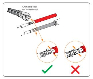
Figure 8-19 Crimping the PV cables with pin contacts
