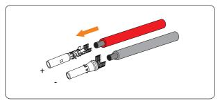
Figure 8-18 Inserting into the PV pin contact
