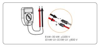
Figure 8-23 Measuring the voltage of PV connectors
