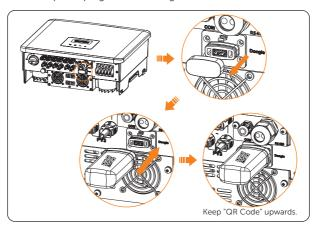
Figure 8-46 WiFi connection procedure
