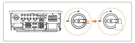
Figure 9-6 Locking the lockable DC switch
