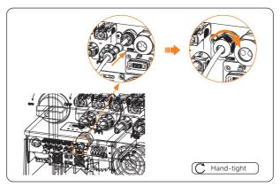
Figure 8-34 Tightening the terminal
