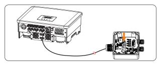
Figure 15-7 Connecting to Adapter Box G2
