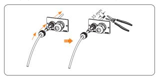
Figure 8-31 Threading and stripping communication cable
