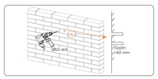
Figure 7-6 Drilling holes
