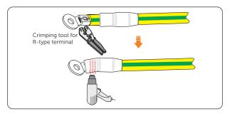
Figure 8-5 Crimping the cable and shrinking the terminal sleeve
