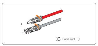
Figure 8-22 Tightening swivel nuts of PV connectors
