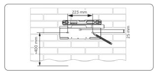
Figure 7-5 Marking the holes
