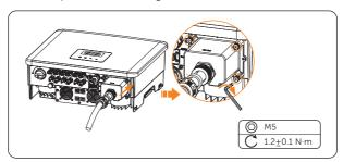
Figure 8-15 Aligning the AC waterproof cover
