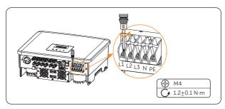
Figure 8-13 Taking down the screws
