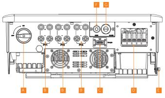
Figure 8-1 Terminals of Inverter
