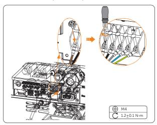
Figure 8-14 Connecting the wires and tightening the screws
