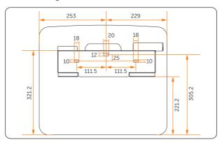
Figure 7-4 Dimensions 2 (Unit: mm)
