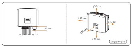
Figure 5-4 Clearance requirement for single inverter
