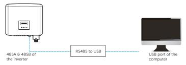
Figure 8-36 Communicating with computer
