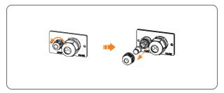
Figure 8-30 Disassembling the COM terminal
