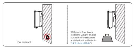
Figure 5-3 Installation carrier requirement
