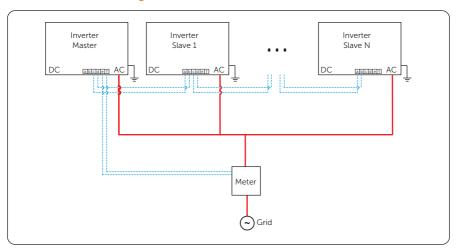
Figure 15-1 Parallel connection with Modbus Function
