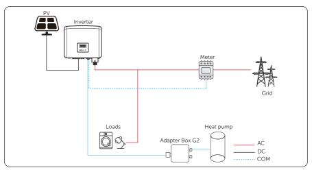
Figure 15-6 Adapter Box G2 wiring diagram
