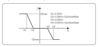
Figure 10-5 Curve Q= f(V)
