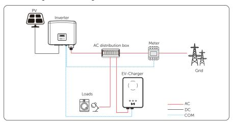
Figure 15-4 EV-Charger wiring diagram
