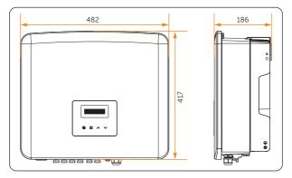
Figure 7-3 Dimensions 1 (Unit: mm)
