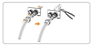
Figure 8-40 Threading and stripping communication cable
