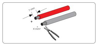
Figure 8-17 Stripping the PV cables
