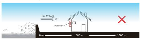
Figure 5-2 Incorrect installation position
