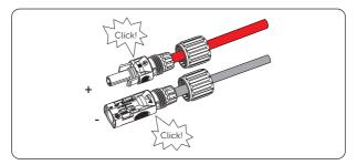
Figure 8-21 Securing the PV cables
