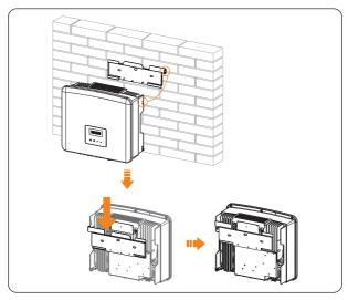
Figure 7-9 Lifting up and hanging the inverter
