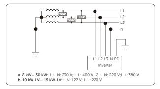
Figure 2-2 Supported power grid - TT
