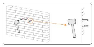
Figure 7-7 Inserting the expansion tubes
