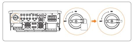
Figure 9-7 Unlocking the lockable DC switch
