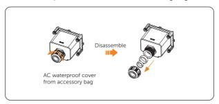
Figure 8-8 Disassembling the AC waterproof cover
