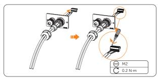
Figure 8-41 Inserting to the terminal block
