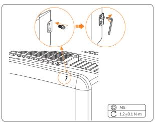
Figure 7-10 Securing the inverter
