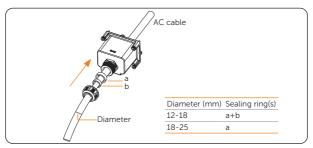
Figure 8-9 Threading the AC cable
