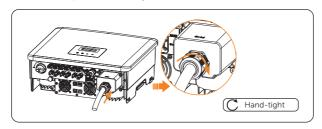
Figure 8-16 Securing the AC waterproof cover
