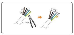
Figure 8-10 Stripping and installing the sleeves
