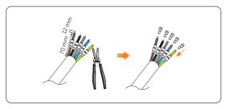
Figure 8-11 Stripping and installing the R-Type terminals
