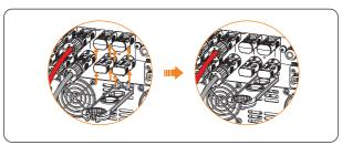
Figure 8-27 Disassembling the dustproof buckles
