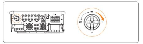
Figure 9-4 Turning on the lockable DC switch
