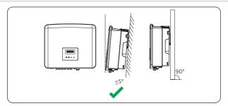
Figure 7-1 Correct installation
