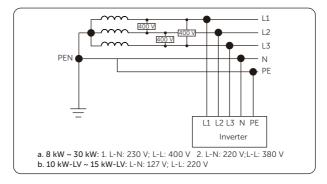
Figure 2-4 Supported power grid - TN-C-S
