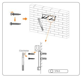
Figure 7-8 Securing the bracket
