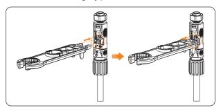
Figure 8-28 Disassembling the PV connectors
