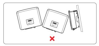
Figure 7-2 Incorrect installation
