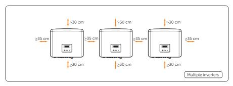
Figure 5-5 Clearance requirement for multiple inverters
