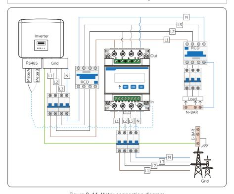
Figure 8-44 Meter connection diagram
