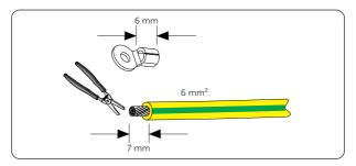
Figure 8-3 Stripping the PE cable
