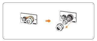
Figure 8-39 Disassembling the RS485 terminal
