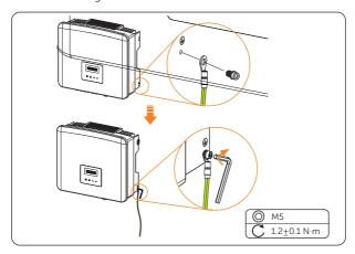
Figure 8-7 Securing the PE cable
