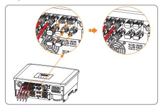
Figure 8-26 Sealing the unused PV terminals
