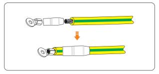
Figure 8-4 Installing the tubing and terminal
