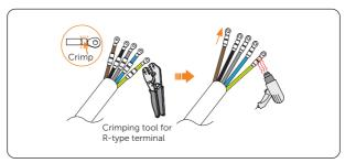
Figure 8-12 Crimping the AC cable end
