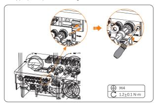
Figure 8-42 Connecting to the inverter
