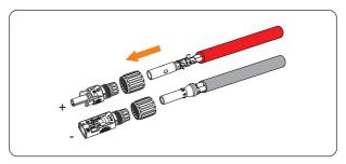
Figure 8-20 Threading the PV cables
