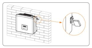
Figure 7-11 Locking the inverter
