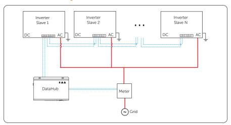
Figure 15-2 Parallel connection with DataHub
