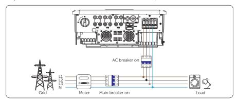
Figure 9-2 Switch on AC breaker
