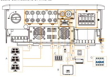
Figure 8-2 Cable connections of inverter
