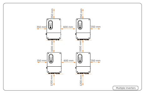
Figure 5-5 Clearance requirement for multiple inverters
