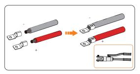
Figure 8-10 Crimping the terminal
