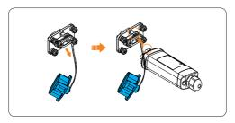
Figure 9-58 Dongle connection procedure
