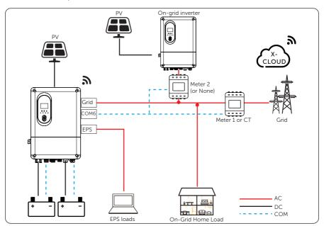
Figure 16-6 AC Couple wiring connection diagram
