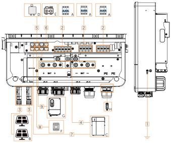
Figure 8-2 Cable connections of inverter
