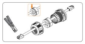
Figure 9-44 Crimping the RJ45
