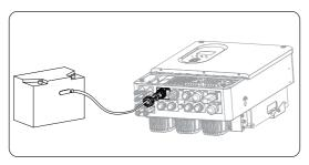
Figure 9-39 Connecting the NTC
