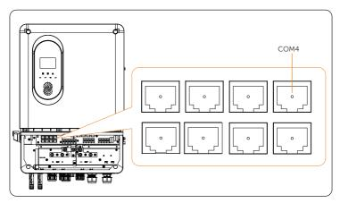
Figure 16-2 Connection terminal for generator
