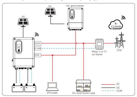
Figure 16-8 Micro-grid (On-EPS terminal)
