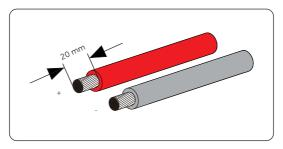
Figure 8-9 Stripping the battery cable
