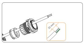
Figure 9-49 Threading the cable
