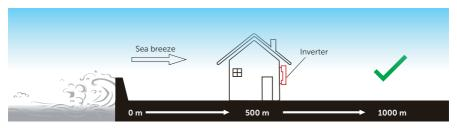
Figure 5-1 Recommended installation position
