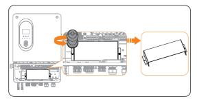
Figure 8-8 Remove the protective cover
