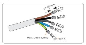
Figure 8-16 Installing the tubing and OT terminal
