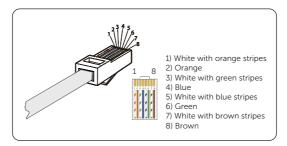
Figure 9-34 Crimping the communication cable
