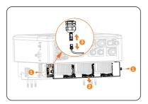
Figure 13-2 Disconnecting the fan
