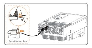
Figure 9-47 Meter connection diagram
