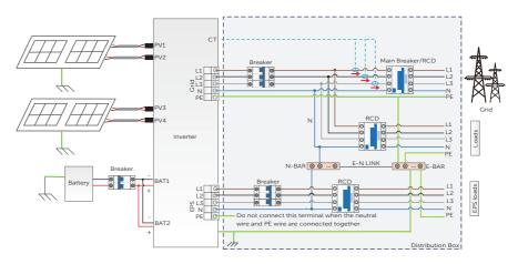
Figure 2-8 Neutral point connected to PE in distribution box
