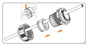
Figure 9-32 Threading the cable
