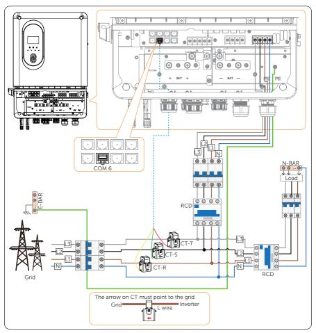
Figure 9-41 CT connection diagram
