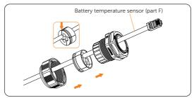
Figure 9-38 Threading the NTC
