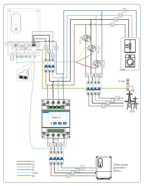
Figure 16-11 Connection diagram of CT and direct-connected meter
