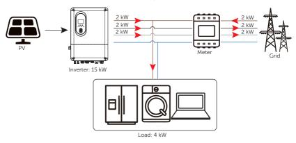
Figure 2-16 Zero grid control with Phase Unbalance disabled
