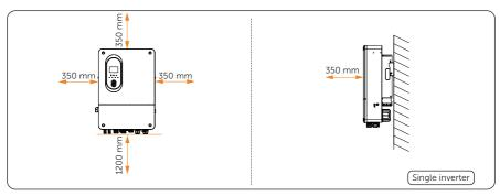
Figure 5-4 Clearance requirement for single inverter
