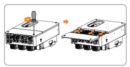
Figure 8-7 Removing the upper cover
