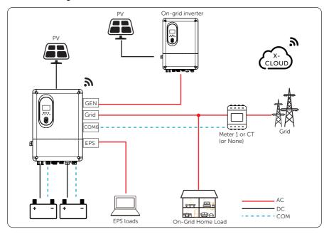
Figure 16-9 Micro-grid (On-GEN terminal)
