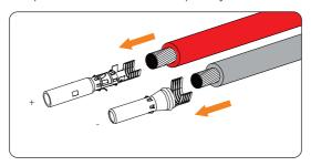
Figure 8-24 Inserting the PV pin contact
