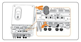
Figure 8-11 Threading the battery cable
