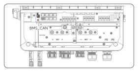
Figure 9-40 Switch on the dip switch
