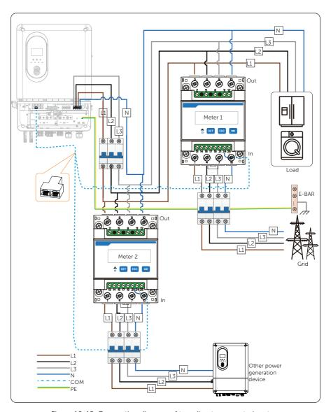
Figure 16-10 Connection diagram of two direct-connected meters
