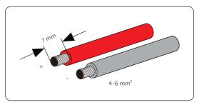
Figure 8-23 Stripping the PV cable
