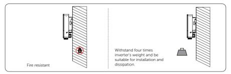
Figure 5-3 Installation carrier requirement
