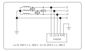
Figure 2-2 Supported power grid-TT
