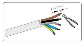
Figure 8-15 Strip the insulation
