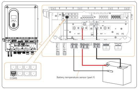
Figure 9-37 Battery temperature sensor connection diagram
