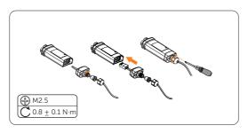
Figure 9-60 Assembling the dongle
