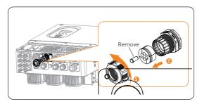
Figure 9-48 Removing the swivel nut
