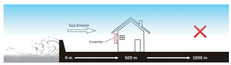
Figure 5-2 Incorrect installation position
