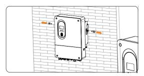
Figure 14-5 Unscrewing the M6 screws
