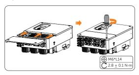
Figure 9-53 Install the upper cover
