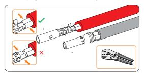
Figure 8-25 Crimping the terminal
