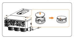
Figure 9-54 Install the upper cover
