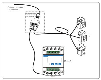
Figure 16-13 Connecting to RJ45 splitter adapter
