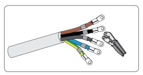
Figure 8-17 Crimping the cable
