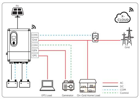
Figure 16-1 Dry contact wiring diagram
