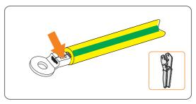
Figure 8-5 Crimping the cable
