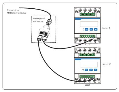
Figure 16-12 Connecting to RJ45 splitter adapter
