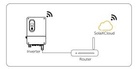
Figure 9-56 LAN mode connection diagram
