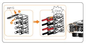
Figure 8-29 Connecting the PV cable
