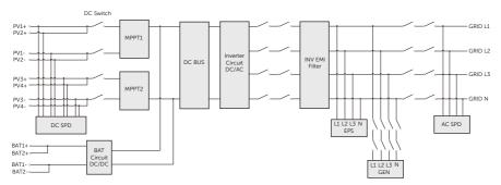
Figure 2-5 Circuit Diagram for X3-NEO-LV series inverter
