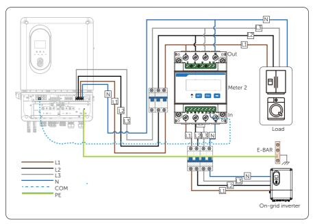
Figure 16-7 Connection diagram of Meter 2 on Grid terminal
