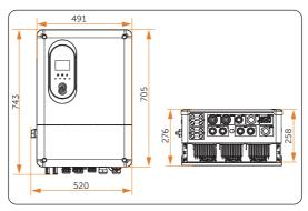
Figure 7-3 Dimensions 1 (Unit: mm)
