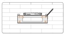
Figure 7-5 Marking the holes
