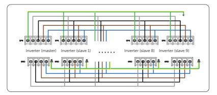
Figure 16-4 Power cable wiring
