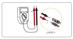
Figure 8-28 Measuring the voltage of PV connectors
