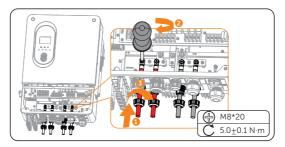
Figure 8-12 Connecting the battery cables
