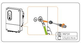
Figure 8-6 Securing the PE cable
