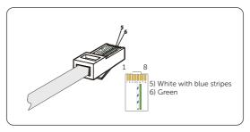
Figure 9-50 Crimping the communication cable
