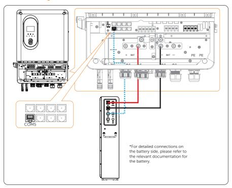
Figure 9-30 BMS connection diagram
