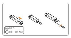
Figure 9-57 Assembling the dongle
