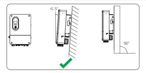
Figure 7-1 Correct installation
