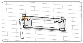
Figure 7-8 Securing the wall mounting bracket
