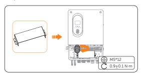
Figure 8-13 Reinstall the protective cover
