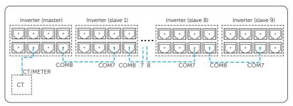
Figure 16-5 Communication cable wiring
