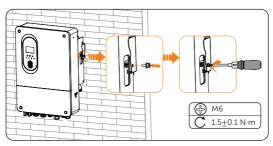
Figure 7-10 Securing the inverter (Right side)
