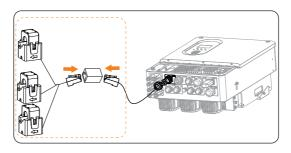
Figure 9-45 CT connection diagram
