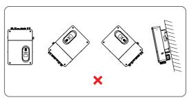
Figure 7-2 Incorrect installation
