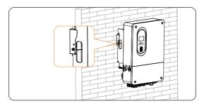
Figure 7-11 Securing the inverter (Left side)
