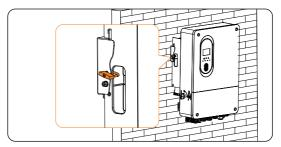
Figure 7-12 Locking the inverter
