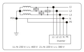
Figure 2-4 Supported power grid-TN-C-S
