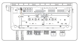
Figure 9-52 Switch on the dip switch
