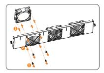
Figure 13-3 Replacing the fan
