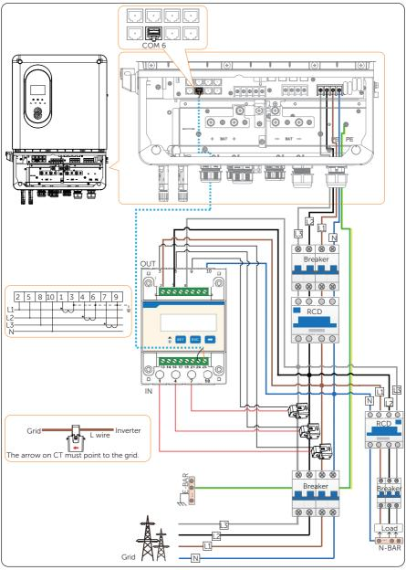
Figure 9-42 Meter connection diagram
