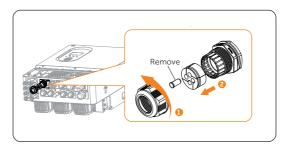
Figure 9-31 Disassembling the connector
