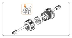
Figure 9-51 Threading the parallel network cable
