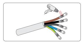
Figure 8-18 Shrinking the tubing
