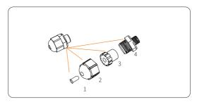
Figure 9-59 Disassembling the waterproof connector
