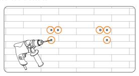
Figure 7-6 Drilling holes
