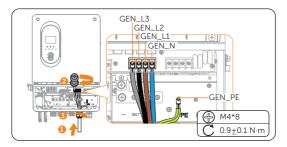
Figure 8-21 GEN terminal connection
