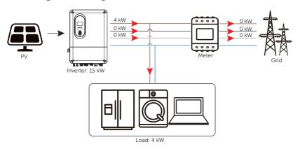
Figure 2-17 Zero grid control with Phase Unbalance enabled
