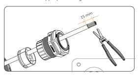
Figure 9-33 Stripping the insulation
