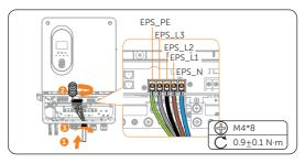
Figure 8-22 EPS terminal connection
