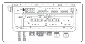
Figure 9-36 Switch on the dip switch
