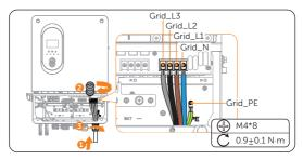
Figure 8-20 Grid terminal connection
