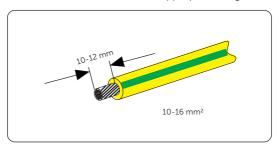
Figure 8-3 Striping the PE cable
