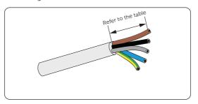
Figure 8-14 Stripping the cable
