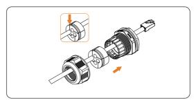
Figure 9-46 Threading the cable
