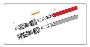
Figure 8-26 Threading the PV cable
