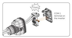
Figure 8-49 Inserting the connector to COM 1
