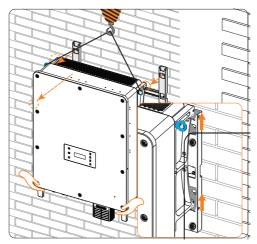
Figure 12-8 Lifting down the inverter
