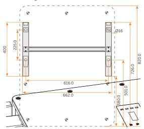
Figure 7-4 Bracket dimensions (unit: mm)
