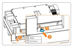
Figure 7-16 Installing the eye bolts
