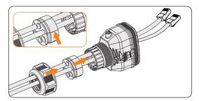
Figure 8-45 Threading the cables with RJ45 terminal
