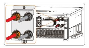
Figure 8-42 Well connected battery cables
