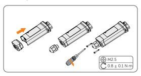
Figure 8-76 Assembling the dongle
