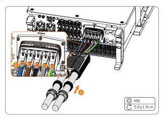
Figure 8-18 Connecting the Grid cable
