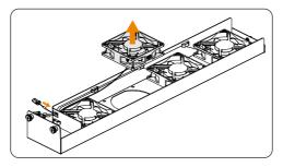
Figure 11-7 Remove the damaged fan
