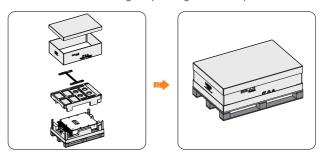
Figure 12-9 Packing the inverter
