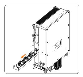
Figure 11-3 Pulling put the whole fan bracket
