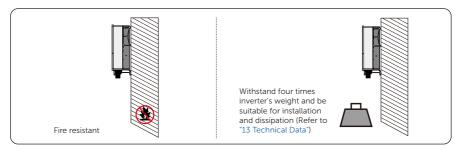
Figure 5-3 Installation carrier requirement
