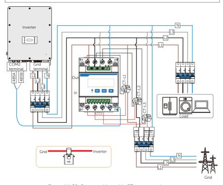
Figure 14-29 System wiring with CT-connected meter
