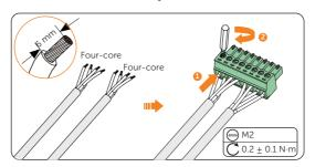
Figure 8-72 Connecting to 8-pin terminal block
