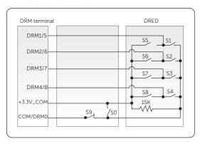
Figure 8-57 DRED connection diagram
