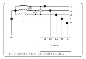
Figure 2-4 Supported power grid-TN-C-S
