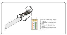
Figure 8-55 Crimping the communication cable
