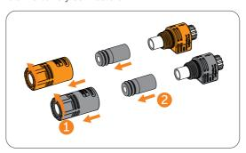
Figure 8-34 Disassembling battery connectors
