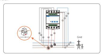
Figure 14-30 Connecting CT-connected meter to the grid
