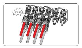
Figure 8-28 Connecting assembled PV cables to the inverter
