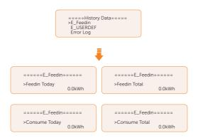
E\_USERDEF: The output electricity of the connected on-grid inverter totay and the total.(detected by Meter 2) This function is only available when meter 2 is connected.
