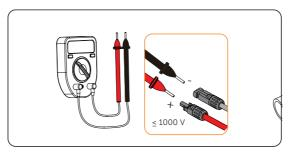
Figure 8-26 Measuring the voltage of PV connectors
