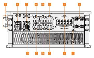
Figure 8-1 Terminals of Inverter
