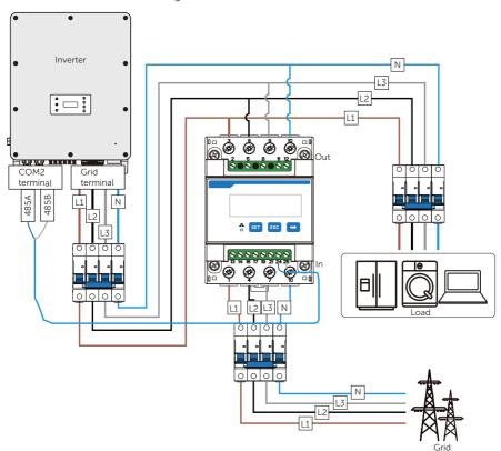
Figure 14-24 System wiring with direct-connected meter
