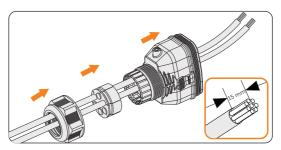
Figure 8-46 Threading the cables and striping the insulation
