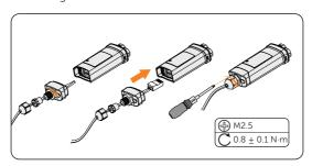
Figure 8-79 Assembling the LAN dongle
