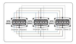
Figure 14-17 Power cable wiring without X3-PBOX-300kW
