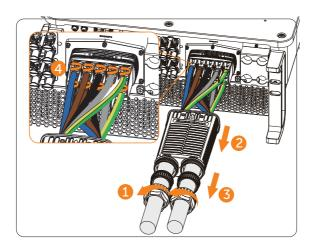
Figure 12-5 Removing AC terminals
