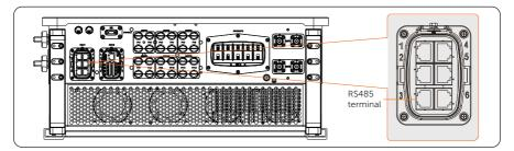
Figure 14-5 Connection terminal for Adapter Box
