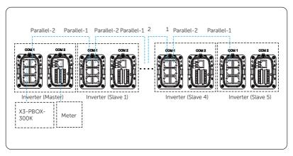
Figure 14-18 Communication wiring with X3-PBOX-300kW
