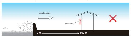
Figure 5-2 Incorrect installation position
