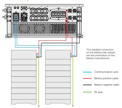
Figure 8-51 BMS connection diagram
