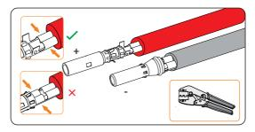
Figure 8-23 Crimping the terminal
