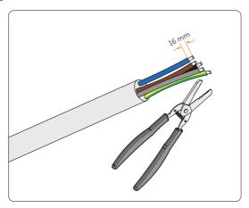
Figure 8-11 Stripping cables
