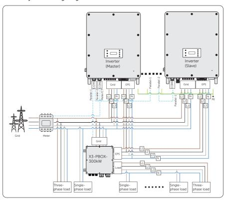
Figure 14-14 With X3-PBOX-300kW system wiring diagram
