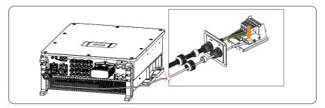
Figure 14-9 Connecting to EV-Charger
