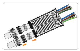
Figure 8-14 Threading cables through the AC connector
