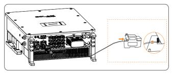
Figure 14-27 Connecting inverter to meter
