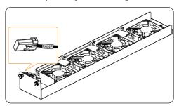
Figure 11-4 Identify the fan to be replaced
