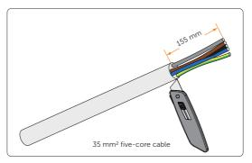
Figure 8-8 Striping the Grid cable
