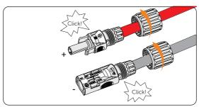
Figure 8-25 Securing the PV cable
