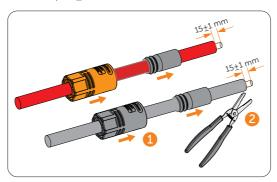
Figure 8-35 Stripping the battery power cable
