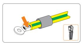
Figure 8-4 Crimping the cable
