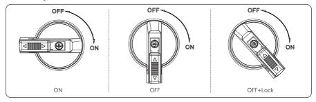
• Turn on the DC switch: rotate the DC switch from OFF state to ON state.
