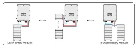
Figure 8-31 Inverter with split battery modules
