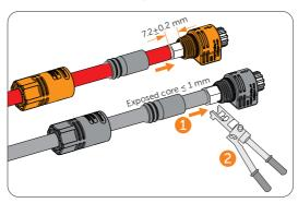
Figure 8-36 Crimping the terminal
