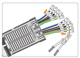
Figure 8-16 Crimping AC terminals
