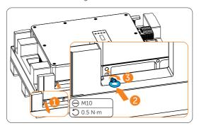
Figure 7-9 Installing the eye bolts
