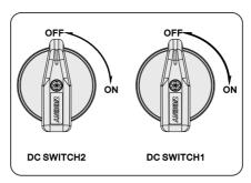
Figure 12-1 Turning off the DC switch
