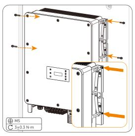
Figure 7-20 Securing the inverter
