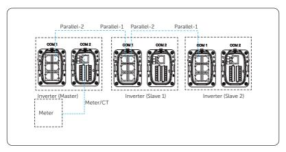
Figure 14-19 Communication wiring without X3-PBOX-300kW
