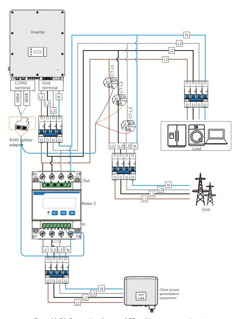
Figure 14-34 Connection diagram of CT and direct-connected meter
