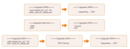
After the upgrade is completed, the LCD screen displays Upgrade Successful. If the upgrades fail, the LCD screen displays Upgrade failed.
