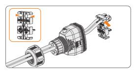
Figure 8-48 Installing the cable to the cable fixture
