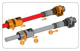
Figure 8-37 Tightening the battery connector
