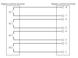
Figure 8-65 Connection diagram for ripple control
