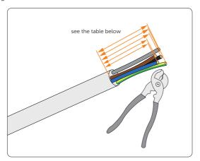
Figure 8-10 Triming cables of the Grid and EPS cable
