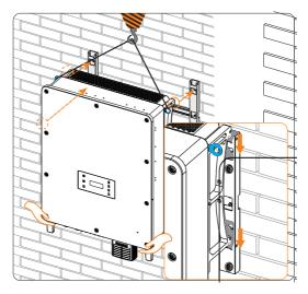
Figure 7-11 Hooking the inverter on the bracket
