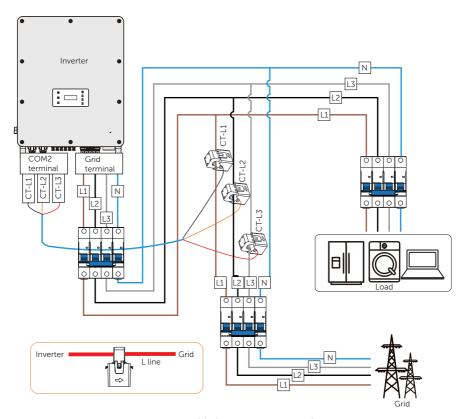
Figure 14-20 System wiring with CT
