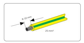
Figure 8-2 Striping the PE cable
