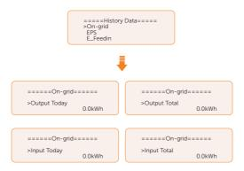
• **EPS**: A record of the output electric energy of the inverter totay and the total. when it is disconencted from grid. (through **EPS** terminal)
