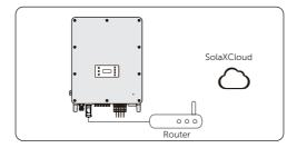
Figure 8-75 LAN mode connection diagram
