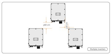
Figure 5-6 Clearance requirement for multiple inverters
