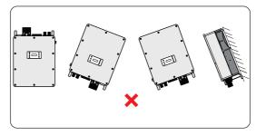
Figure 7-2 Incorrect installation
