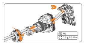
Figure 8-50 Securing the connector
