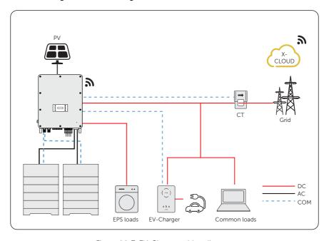
Figure 14-7 EV-Charger wiring diagram
