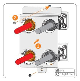
Figure 8-41 Installing the battery proctective cover
