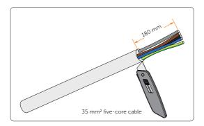
Figure 8-9 Striping the EPS cable
