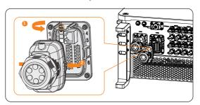
Figure 8-59 Disassembling the COM 2 terminal
