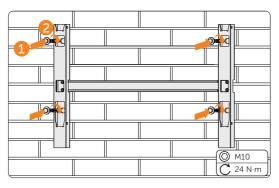
Figure 7-8 Securing the mounting bracket
