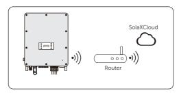
Figure 8-74 Wi-Fi mode connection diagram
