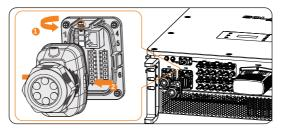
Figure 8-66 Disassembling the COM 2 terminal
