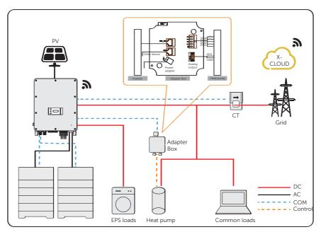
Figure 14-4 Adapter Box wiring diagram
