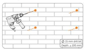
Figure 7-7 Drilling holes
