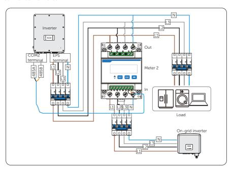
Figure 14-13 Connection diagram of Meter on EPS terminal
