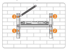
Figure 7-6 Marking the rest holes
