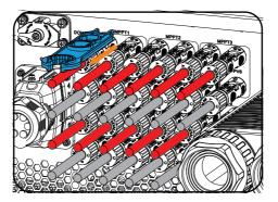
Figure 12-2 Releasing the PV connector
