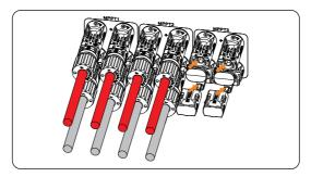
Figure 8-29 Installing PV dustproof buckles
