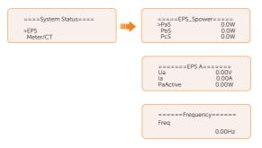
Meter/CT status: Information contains feed-in power of L1, L2 and L3 detected by the connected meter or CT.
