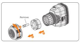
Figure 8-67 Disassembling the connector
