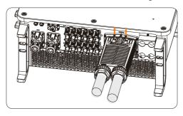
Figure 12-4 Removing AC connector
