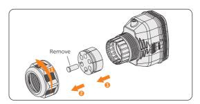
Figure 8-53 Disassembling the connector
