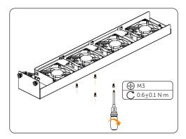
Figure 11-9 Lock the screws
