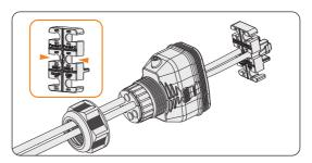
Figure 8-52 Installing RJ45 terminal to the cable fixture
