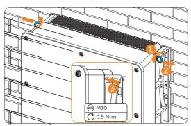
Figure 7-12 Removing the eye bolts
