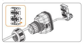
Figure 8-58 Installing RJ45 terminal to the cable fixture
