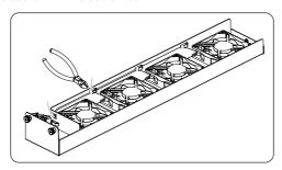
Figure 11-10 Unscrew the fan screws
