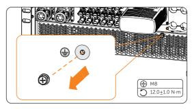
Figure 8-6 Uninstalling the screw
