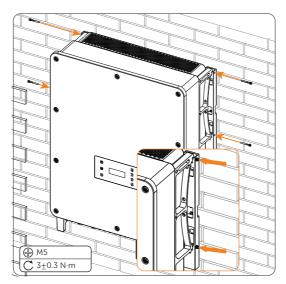
Figure 7-13 Securing the inverter
