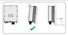
Figure 7-1 Correct installtion
