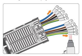
Figure 8-17 Shrinking the tubings
