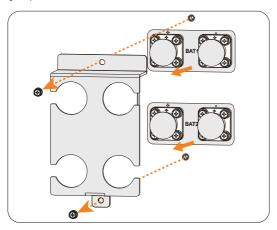
Figure 8-38 Removing the battery protective cover
