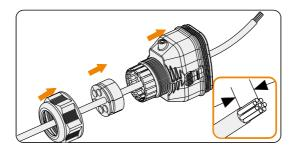
Figure 8-54 Threading the cables and striping the insulation
