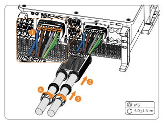
Figure 8-19 Connecting the EPS cable
