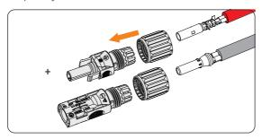
Figure 8-24 Threading the PV cable
