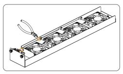
Figure 11-5 Cut the cable ties
