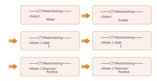
Figure 14-37 Selecting meter and set Meter 1 and Meter 2 data
