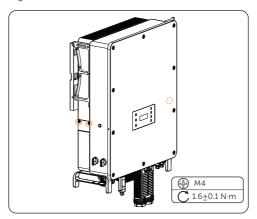
Figure 11-13 Lock the screws
