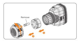
Figure 8-44 Disassembling the connector
