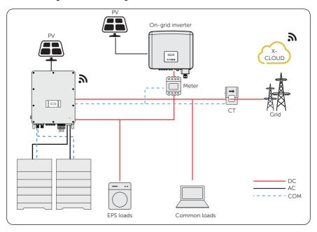
Figure 14-10 Micro-grid wiring connection
