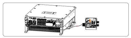
Figure 14-6 Connecting to Adapter Box
