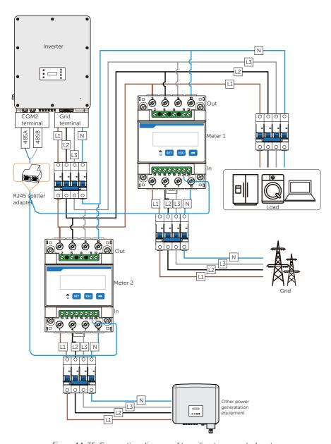
Figure 14-35 Connection diagram of two direct-connected meters
