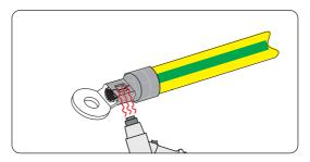
Figure 8-5 Shrinking the tubing
