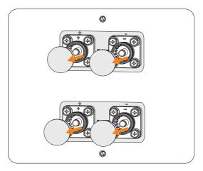
Figure 8-39 Removing battery caps
