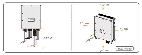
Figure 5-4 Clearance requirement for single inverter
