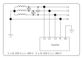
Figure 2-2 Supported power grid-TT
