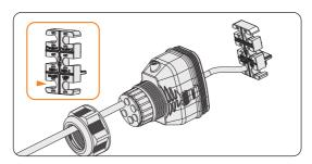
Figure 8-56 Installing RJ45 terminal to the cable fixture
