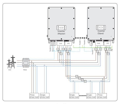
Figure 14-15 Without X3-PBOX-300kW system wiring diagram
