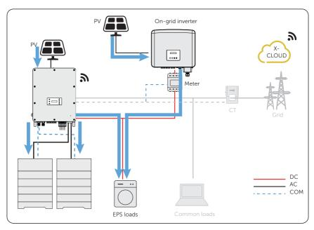
Figure 14-12 Power flowing when grid off
