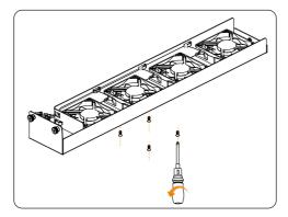
Figure 11-6 Unscrew the fan screws
