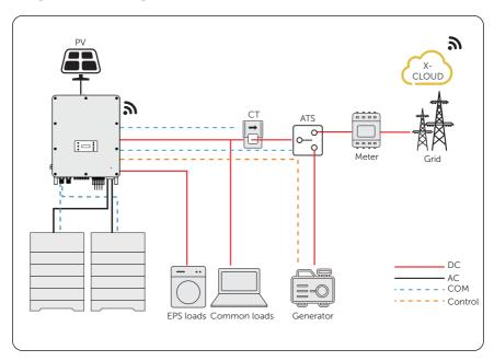
Figure 14-2 Dry contact wiring diagram
