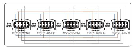
Figure 14-16 Power cable wiring with X3-PBOX-300kW
