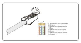
Figure 8-47 Crimping the communication cable
