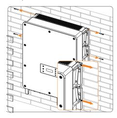
Figure 12-6 Unscrewing screws on the inverter
