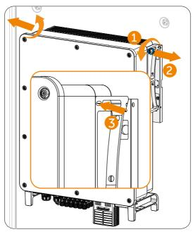
Figure 7-19 Removing the eye bolts
