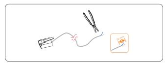
Figure 14-31 Stripping communication cable for meter
