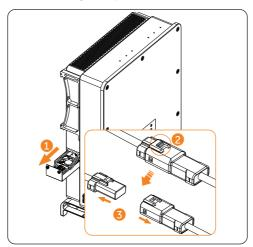
Figure 11-2 Releasing the fan waterproof connectors
