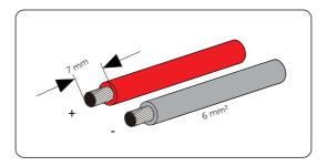
Figure 8-21 Striping the PV cable
