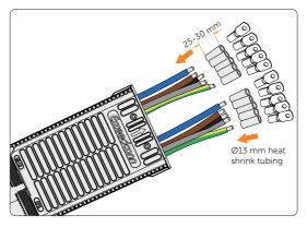
Figure 8-15 Assembling tubings and AC terminals
