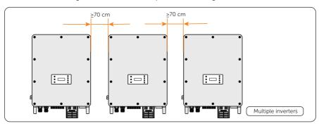
Figure 5-5 Clearance requirement for multiple inverters
