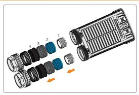
Figure 8-13 Disassembling the swivel nuts
