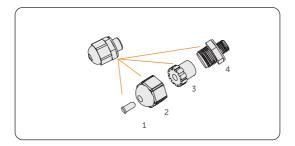
Figure 8-78 Disassembling the waterproof connector
