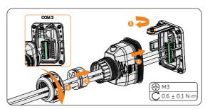
Figure 8-70 Connecting to the inverter
