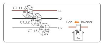
Figure 14-21 Clipping CTs to grid cables
