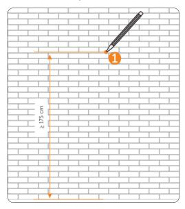
Figure 7-5 Marking the first hole
