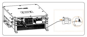
Figure 14-32 Connecting inverter to meter
