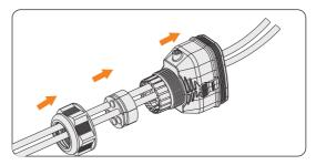
Figure 8-68 Threading the cables
