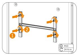
Figure 7-15 Securing the mounting bracket
