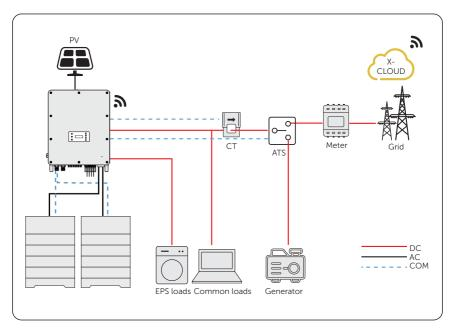
Figure 14-1 ATS control wiring diagram
