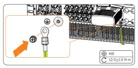
Figure 8-7 Securing the PE cable
