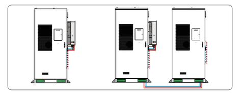
Figure 8-32 Inverter with battery cabinet(s)
