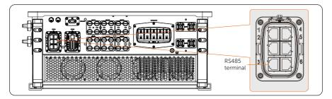
Figure 14-8 Connection terminal for EV-Charger
