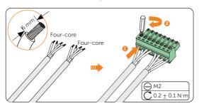
Figure 8-69 Connecting to 8-pin terminal block
