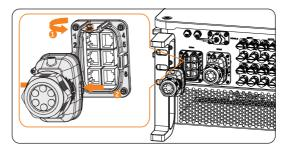
Figure 8-43 Removing the connector enclosure
