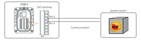
Figure 8-71 System switch connection diagram
