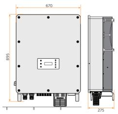
Figure 7-3 Dimensions (unit: mm)
