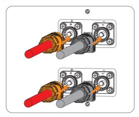
Figure 8-40 Connecting assembled battery cables
