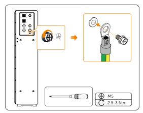
Figure 7-4 Tightening M5 screws
