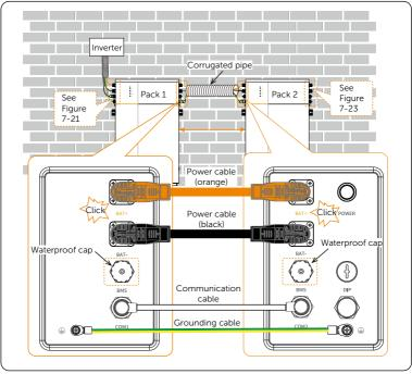
Figure 9-2 Cable connection between adjacent battery pack
