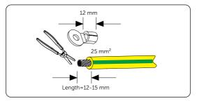
Figure 7-1 Striping cable jacket
