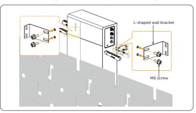
Figure 6-2 Fixing L-shaped wall bracket to the battery pack
