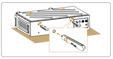
Figure 5-4 Inserting handles
