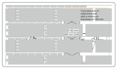
Figure 6-5 Drilling holes
