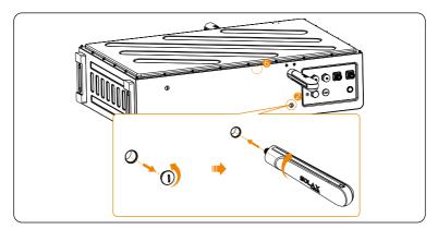
Figure 5-7 Tightening handles
