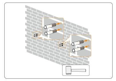
**Step 5:** Insert the expansion bolt (Part G) (x 4 pcs) into the four holes.
