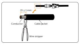
Figure 7-12 Striping cable jacket
