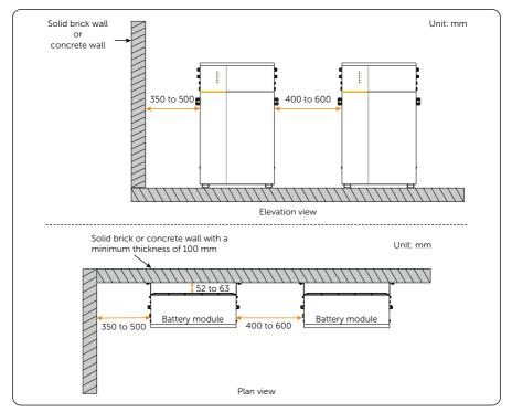
Figure 4-2 Clearance requirement
