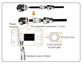
Figure 7-13 Fitting connector body and crimping terminal
