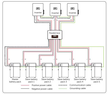
Figure 8-1 Wiring Diagram for Parallel Connection
