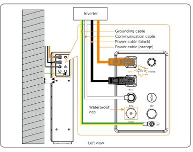
Step 2: Connect the negative power cable to the "BAT-" ports of adjacent battery packs. Connect the positive power cable to the "BAT+" ports of adjacent battery packs. Connect the communication cable to the "BMS" ports of adjacent battery packs.
