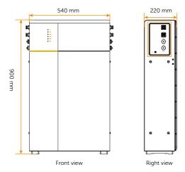
Figure 2-2 Dimension: Battery pack (TP-LD150)
