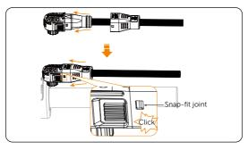
Figure 7-14 Assembling connector
