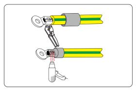
Figure 7-3 Crimping and heating
