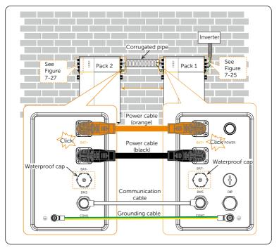
Figure 7-26 Wiring between battery packs
