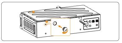
Figure 5-6 Inserting the plastic plug
