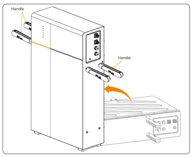
Figure 5-8 Lifting battery pack
