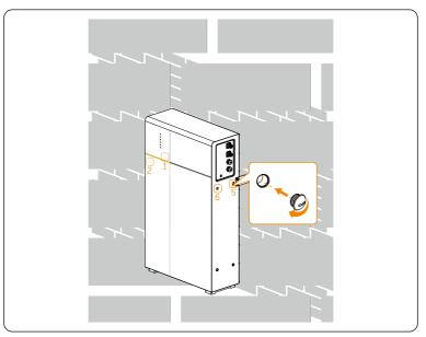
Figure 6-9 Inserting and tightening plastic plugs
