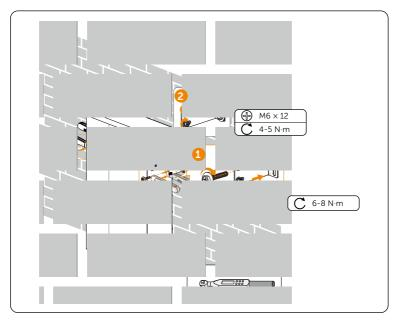
Figure 6-7 Tightening tapping screws and M6 screws
