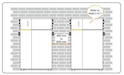
Figure 6-10 Installing the remaining battery pack
