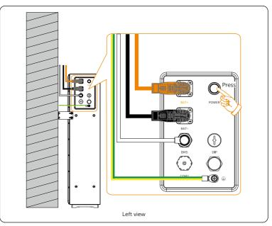
Figure 10-1 Power on/off the system
