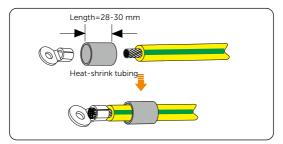
Figure 7-2 Cutting heat-shrink tubing
