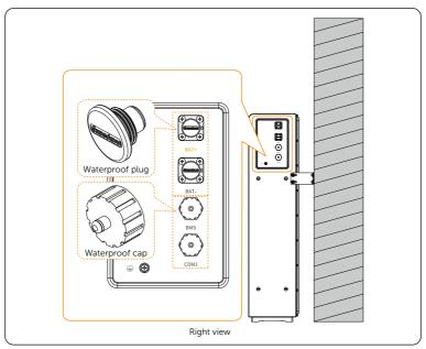
Figure 7-23 Right electrical area of the battery pack
