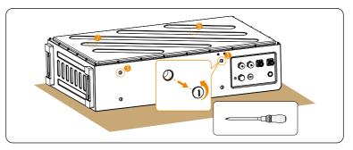
Figure 5-3 Removing plastic plugs
