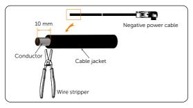
Figure 7-7 Stripping power cable
