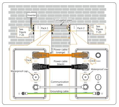
Figure 7-22 Wiring between battery packs
